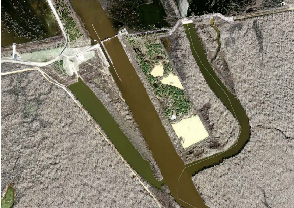
Figure 7. Felsenthal Lock and dam is in the upper center of photo. Brown colored water is the Ouachita River. Channel on left is the boat ramp access channel with confluence at a right angle to the river. The old river channel is directly across the Ouachita River from the boat access channel and is on the right of the photo. If one looks closely the old railroad bridge piers are visible in the old river channel at top next to the channel block which is an extension of the dam.
